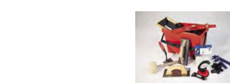
1 Installation of ceramic tiles should be carried out by skilled personnel, with demonstrable experience and appropriate tools and equipment, (i.e. toothed trowels, tile spacers, rubber mallets and suction cups for installation, and rubber trowels, sponges and containers for grouting). Check the information contained on the packaging beforehand, and meticulously follow the manufacturer's recommendations.
